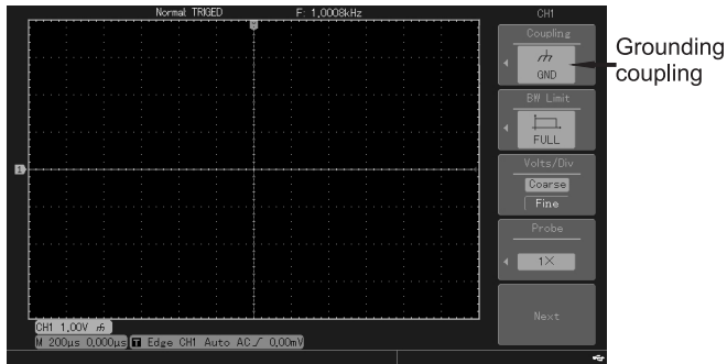
Picture 2-3 channels are being set as grounding
